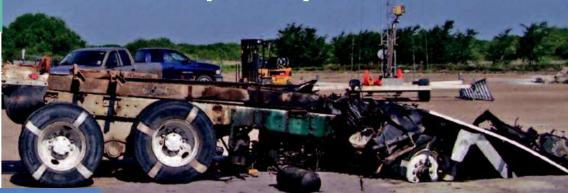
Stop and Destroy a 65,000lb (29,484 kg) vehicle traveling at 50mph (80kph )
